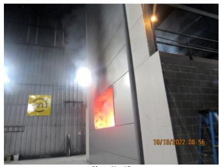
Photo No. 18 Flame tips exiting window opening
