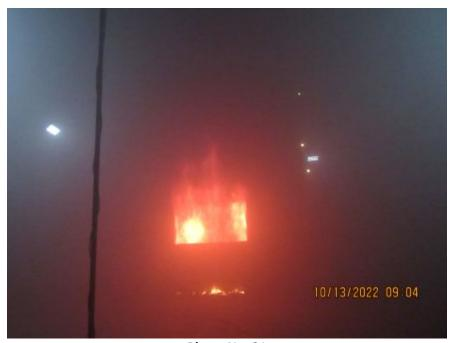
Photo No. 21 Flame increased to 2.5 meters
