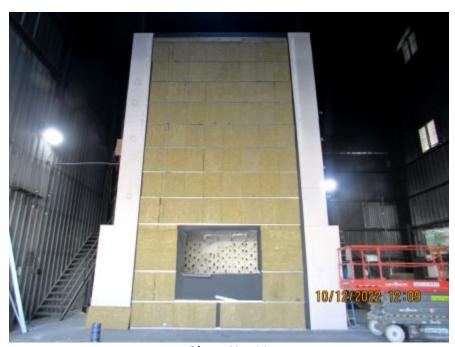
Photo No. 11 Mineral wool installed
