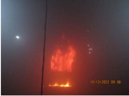
Photo No. 24 Flame height at 4 meters
