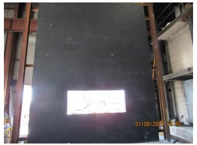
Photo No. 6 Weather Barrier Installed
