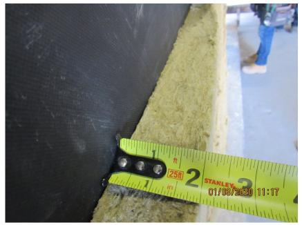
Photo No. 8 Insulation thickness
